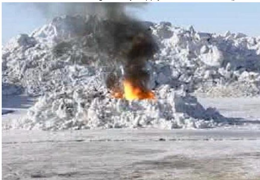
Figure 12: Burning oiled snow, that are piled into a volcano-shaped pile. From Buist et al. (2013), source Alaska Clean Seas.
