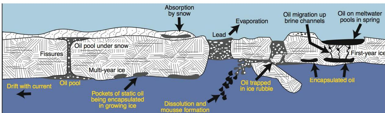
Figure 1: Sketch of oil-in-ice configurations after Al Allen (Dickins 2011).
