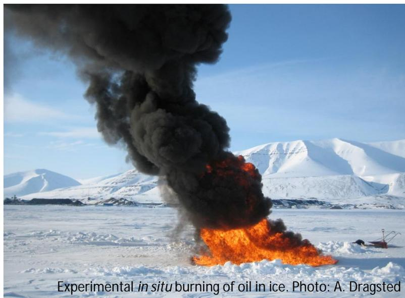
Experimental *in situ* burning of oil in ice. Photo: A. Dragsted
