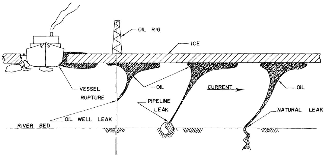
Figure 2: Schematic representation of events which could result in oil spilled beneath sea ice. From Uzuner et al. (1979).
