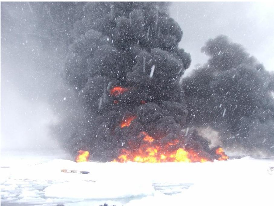
Figure 11: Photograph of the large scale *in situ* burning of oil in broken ice (70-90 %) in the Barents Sea (Photo: J. Fritt-Rasmussen).
