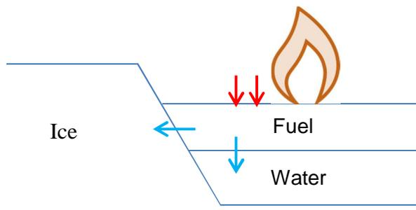
Heat loss: conduction through the sides and bottom →
