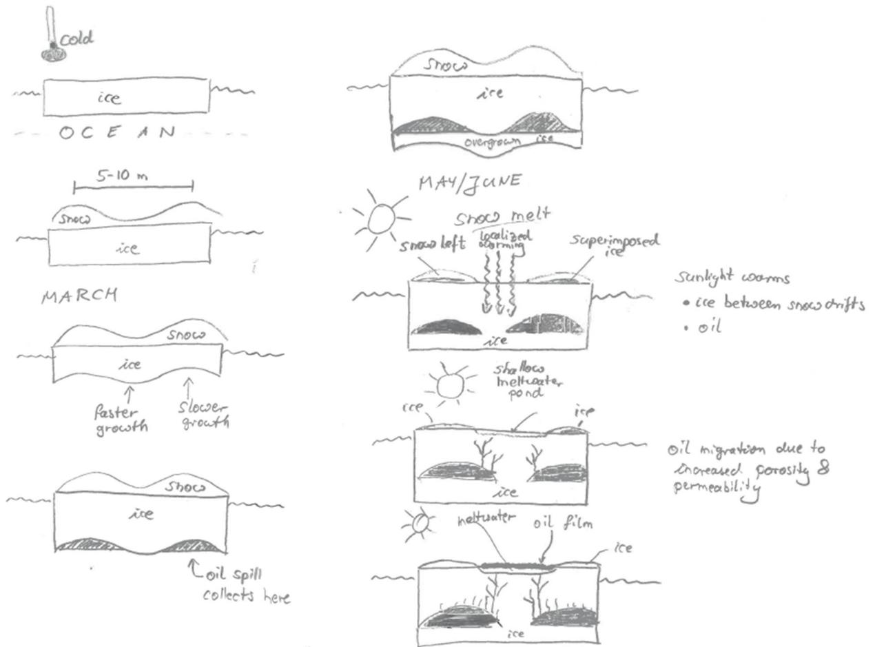
Figure 3: Schematic of the melt process from the perspective of oil.
