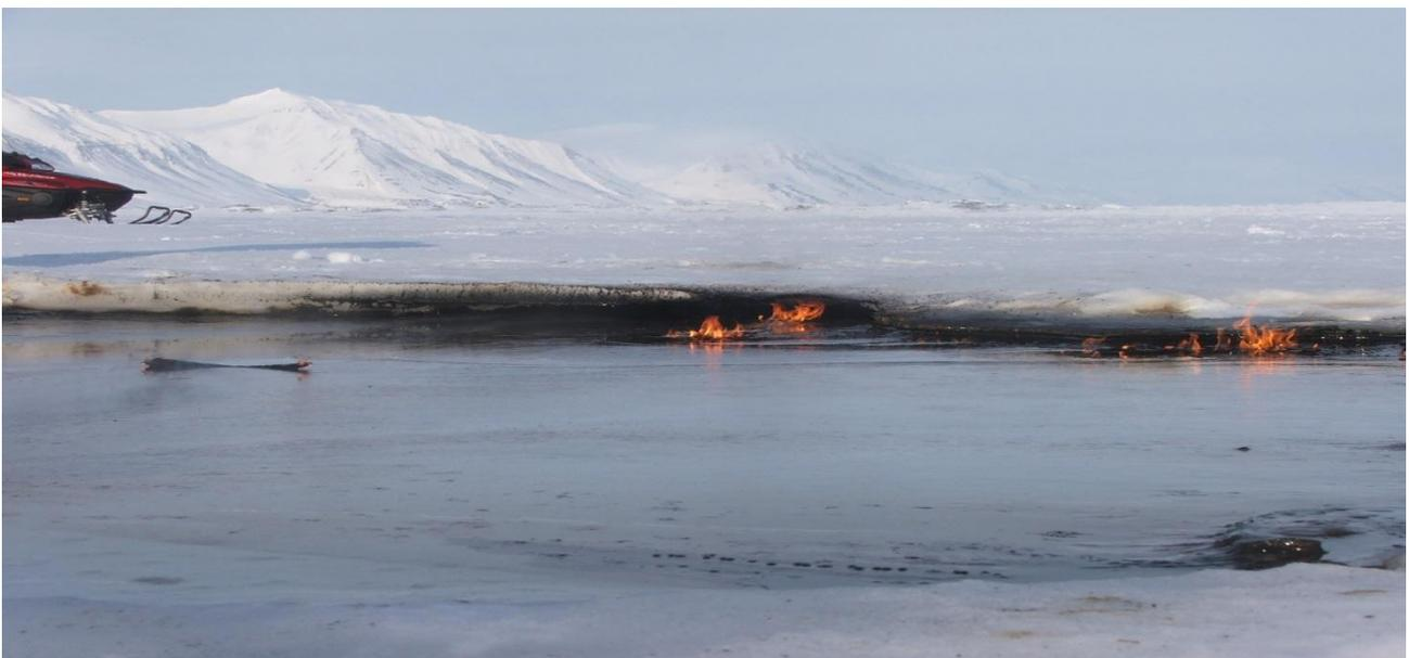
Figure 14: Burning oil on top of the fjord ice on Svalbard. Note that the burning is actually taking place under the snow/ice cover in the lateral ice cavity that was made as a result of the burning of oil. Photograph: J. Fritt-Rasmussen.
