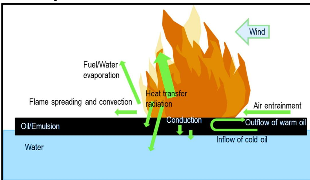
Figure 7: Key heat transfer processes during *in situ* burning operation on water. From Fritt-Rasmussen (2010)
