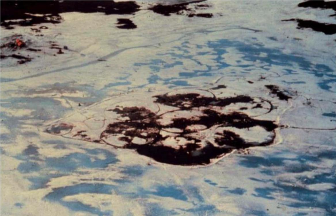
Figure 6: Oil surfacing through sea ice during the pre-melt stage during experiments of NORCOR (1975). Photo from Dickins (2011). Circles are estimated at 10-20 m diameter.
