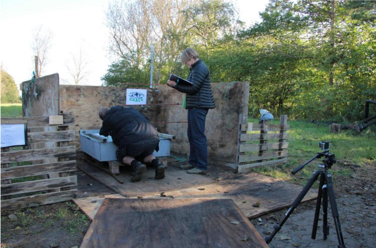
Figure 4. Experiment set-up during dry run on 6 October 2017. The weather station can be seen behind the shelter, slightly to the right of the “Grace” sign. A camera set up to record the burn is seen in the front right of the photo.
