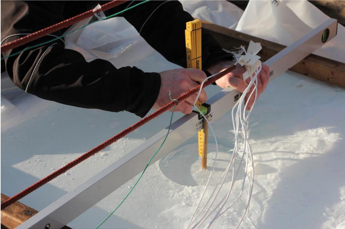
Figure 7. Surface profile measurement before the introduction of oil. Experiment 1 of 15 Nov 2017.
