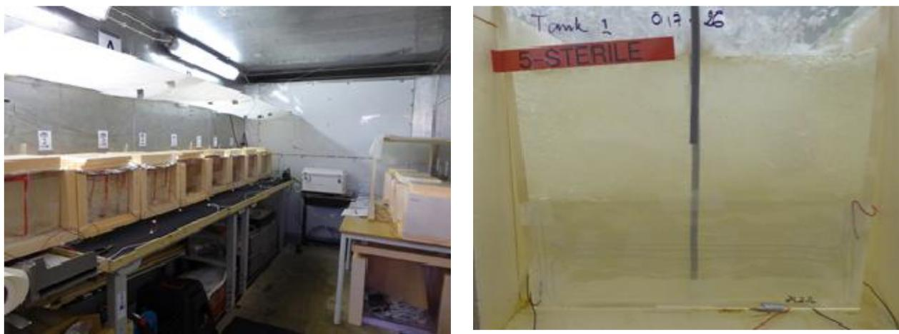
Figure 6. Ice tank mesocosms with water accommodated fractions of dispersed oil (WAF+CE). A. Ice tanks in the cold lab; B. Sterile control tank with water accommodated fractions of dispersed oil.
