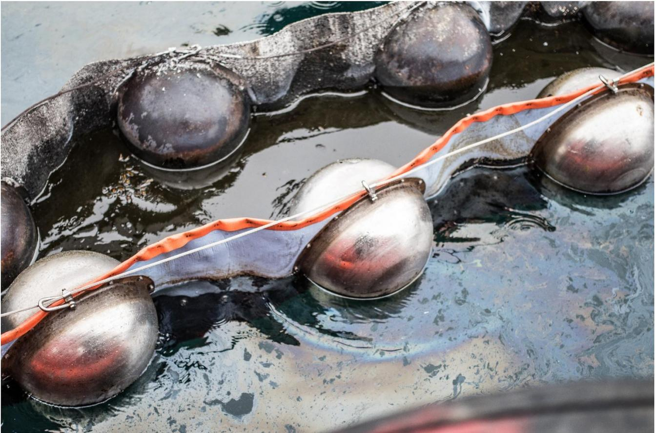
*Figure 2. Picture of Desmi firebooms after termination of both burns*
