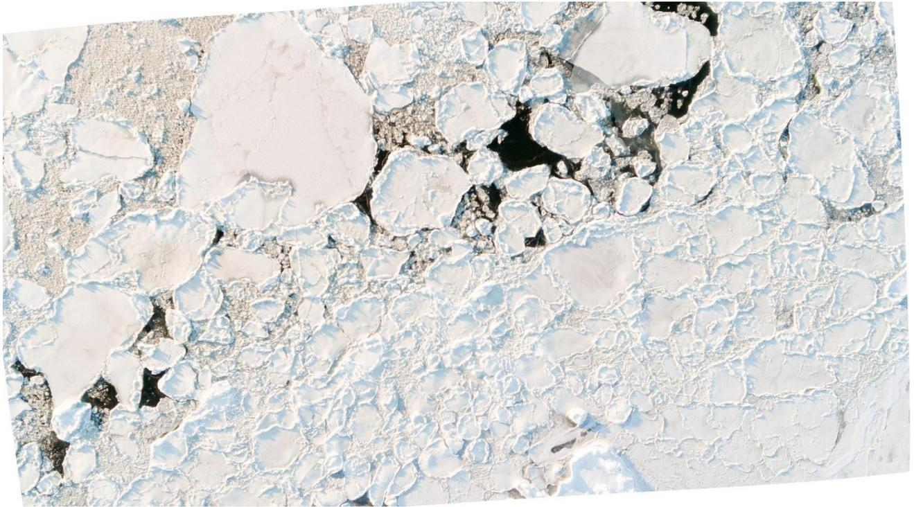
Figure 8 Fine scale structure of the ice field obtained from UAV flight, image taken with down-looking camera, size of ice floes as well open water areas between ice could be well detected
