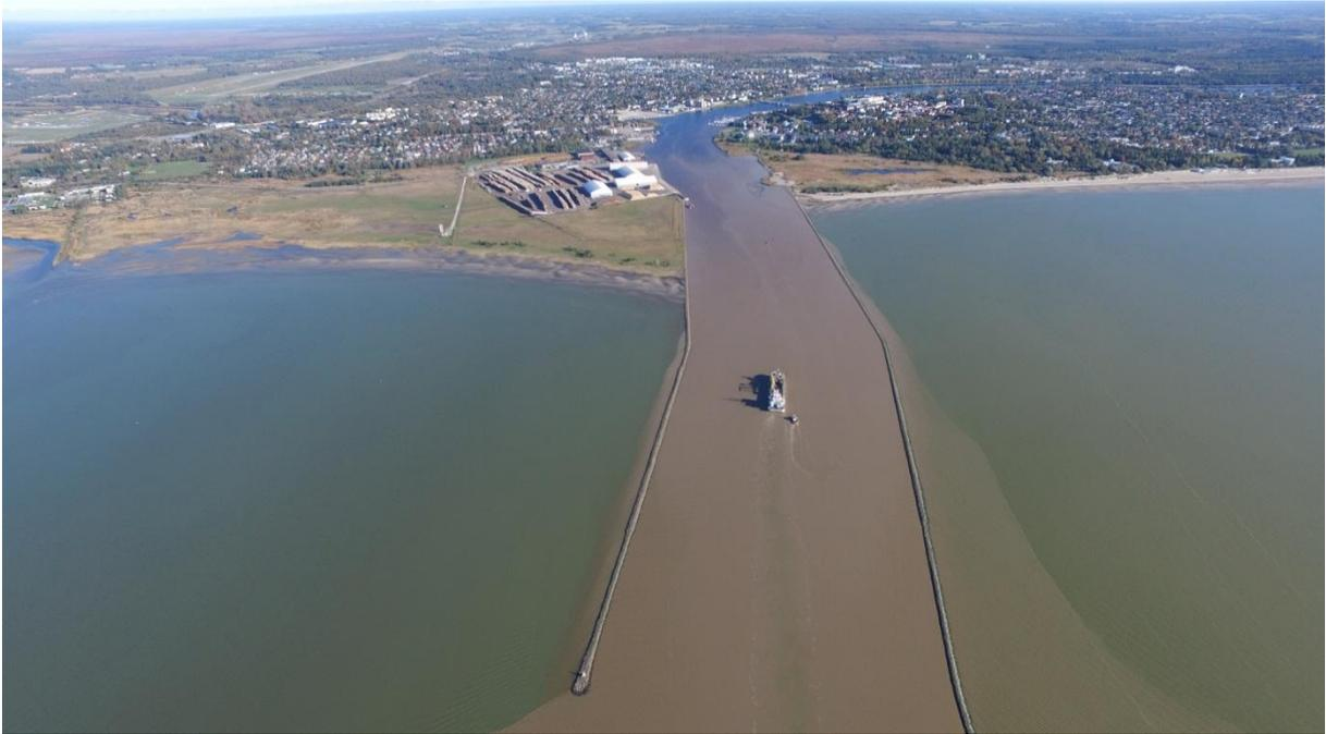
Figure 38 Image showing suspended matter distribution in the dredging zone, dredging vessel between bulwarks, leaving cleaner trail behind what tells that suspended matter is located mainly on surface
