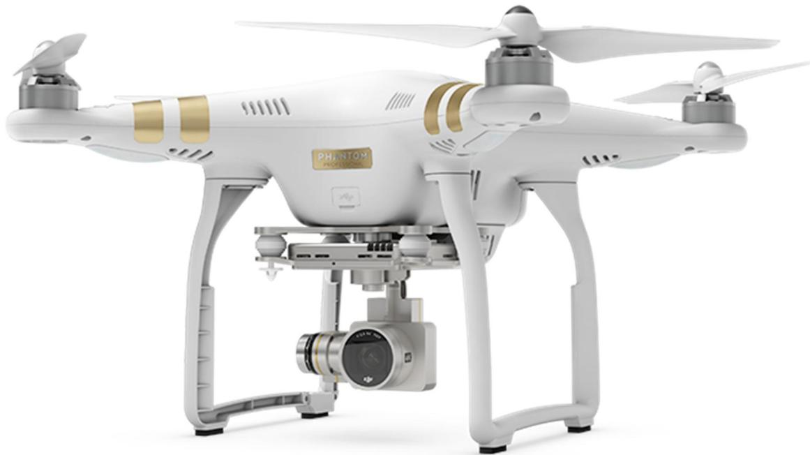
Figure 4 Typical VTOL Mini UAV - DJI Phantom 3 [5]
