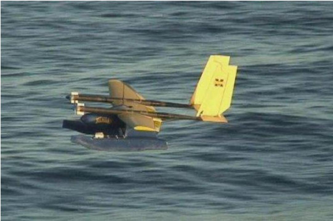
Figure 3 Tactical Unmanned Aerial Vehicle (TUAV) - "Flying Fish" unmanned aircraft takes off and lands on water [4]
