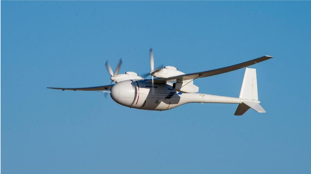
Figure 2 High Altitude/Long Endurance (HALE) UAV - Boeing Phantom Eye [3]
