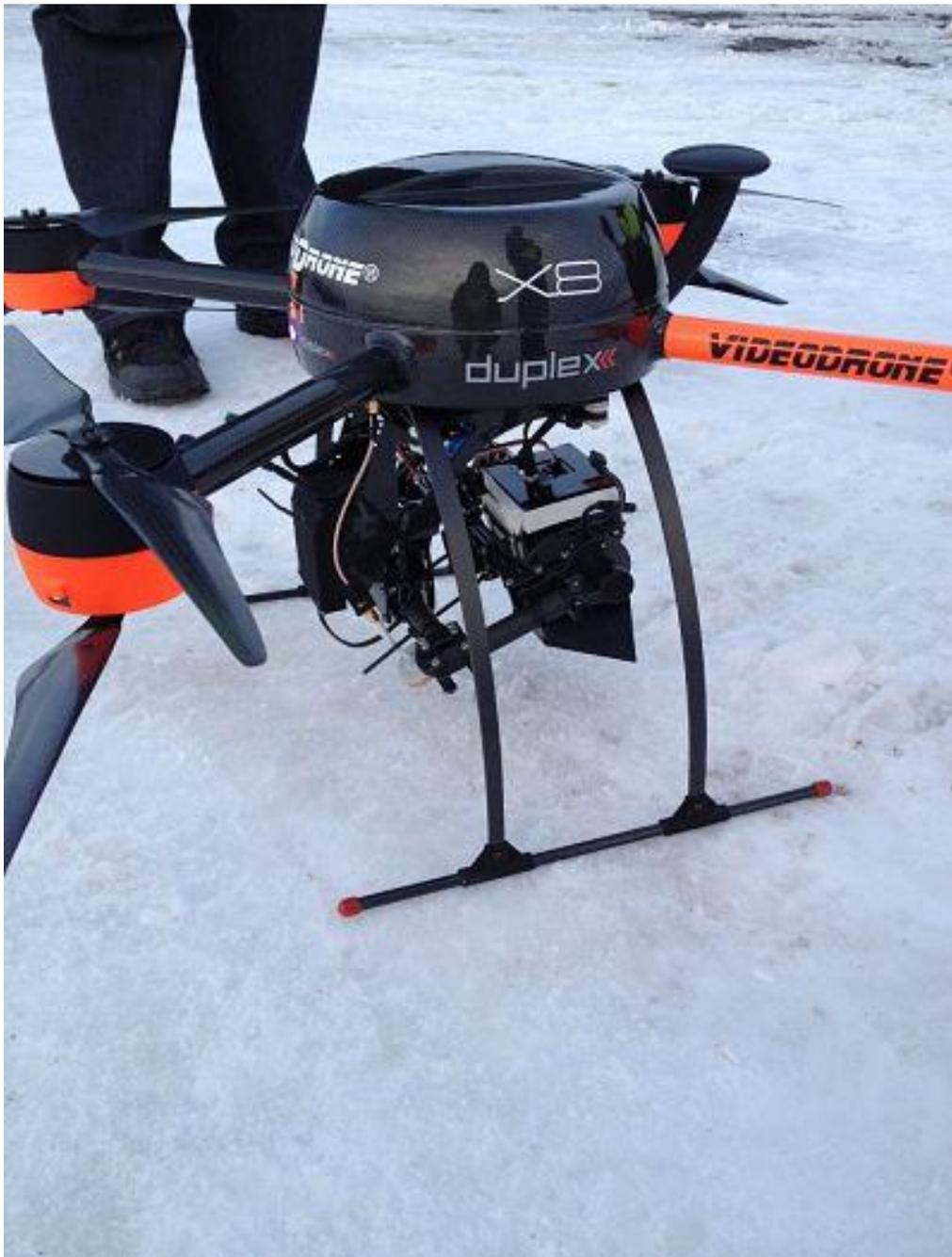
Figure 22 Thermal infrared camera attached to the drone.
