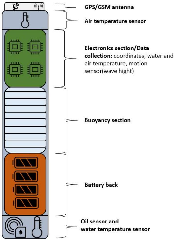
Figure 34 Rough schematics view of the oil detecting drifter buoy prototype.
