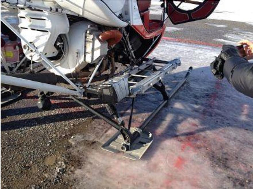
Figure 1 Hyperspectral camera of Jussi Soukkumaki design attached to the copter and ready for uptake.
