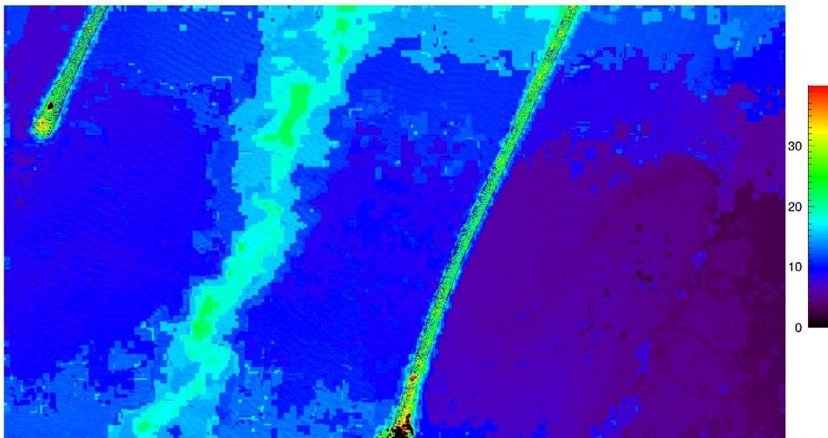
Figure 43 Example of TSM concentration calculated from the image data on 28 October 2015. Measured TSM values varied between 18.0 – 19.2 mg/l, agrees well with buoy data (Fig. 40).
