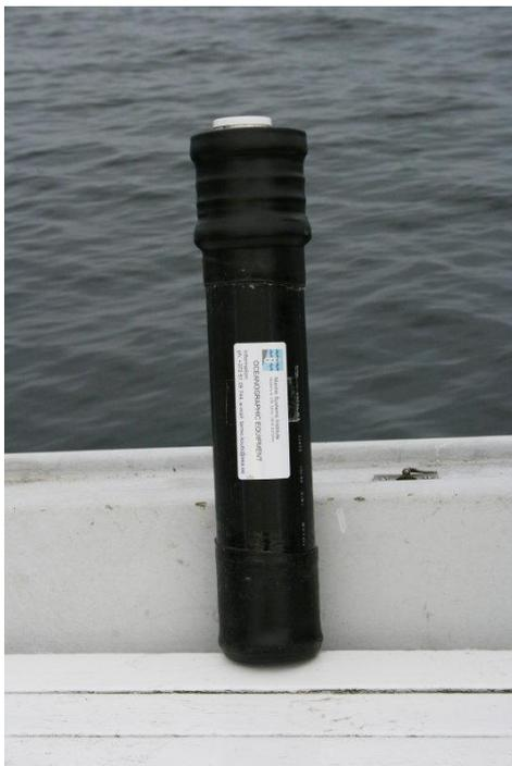
Figure 33 Autonomous drifter buoy developed by Tallinn University of Technology
