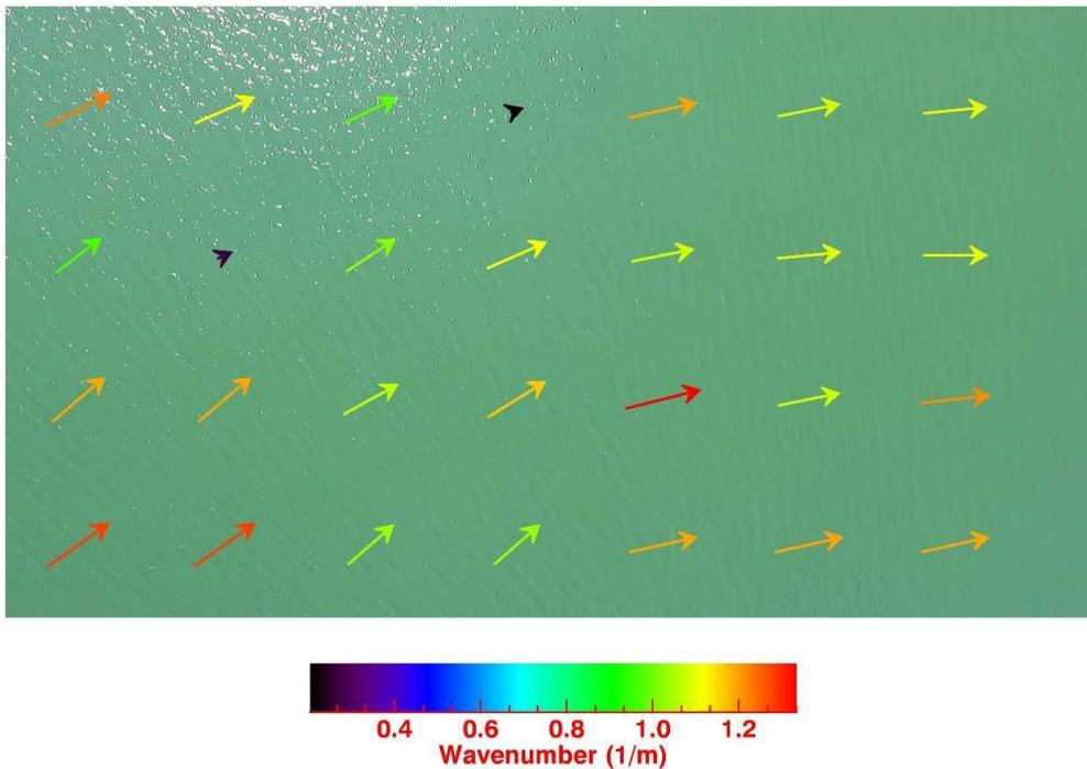
Figure 16 Local wave field obtained from vertically down-looking camera of DJI drone. The Sun light reflected and scattered from the wave slope is recorded by the sensor as glints and different shades of grey (in case if color channels are separated). In principle, a wave passing through a medium does not displace matter horizontally, but as glints form for a given Sun-wave-sensor geometry, the glints
