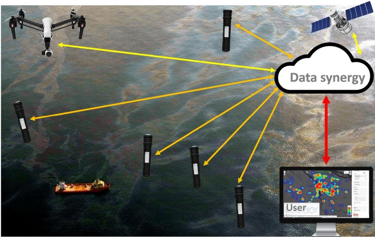
Figure 46 Concept for an on-line/real-time system that combines information from UAVs and drifters (and satellites, if possible), in case of an oil spill
