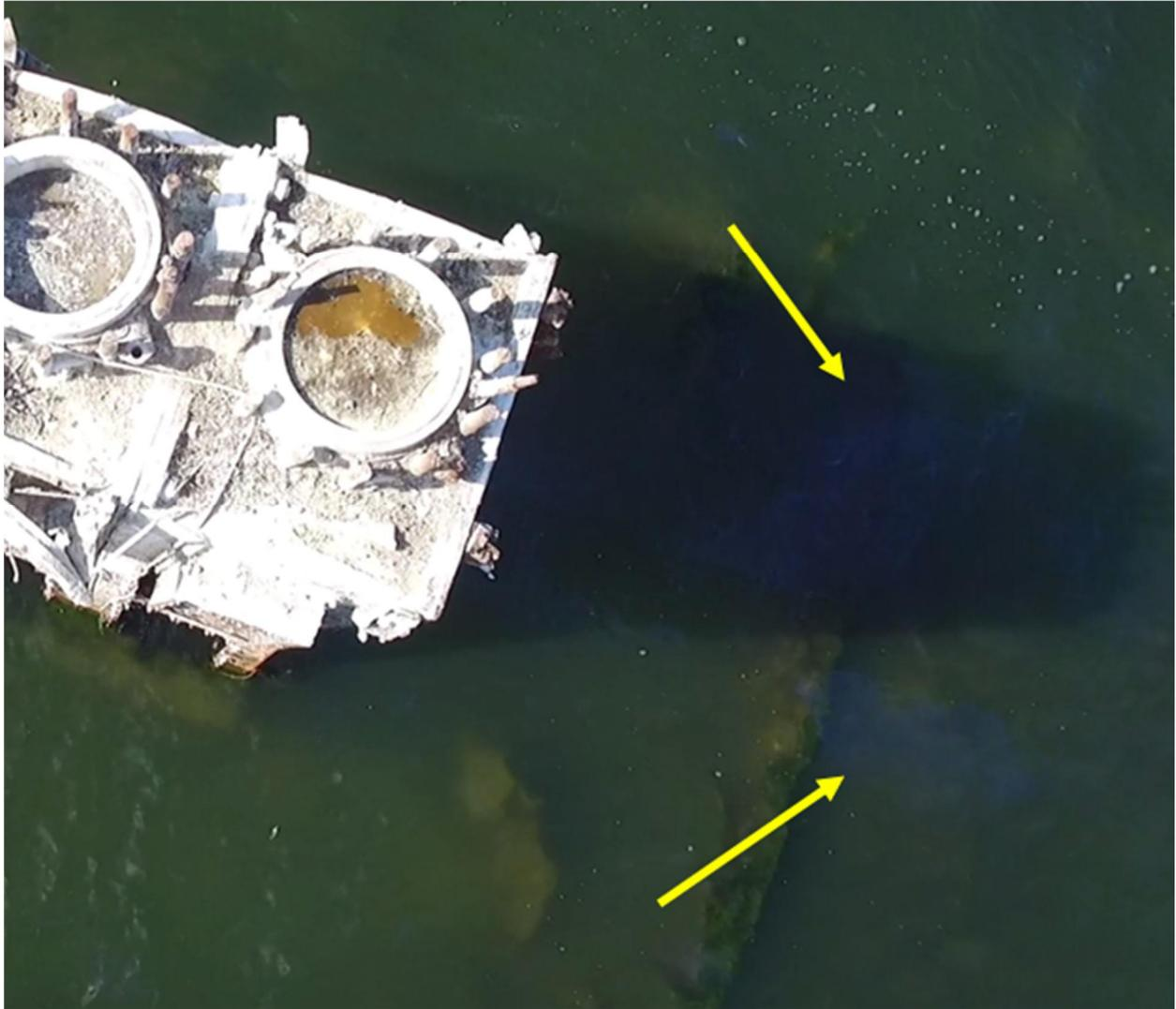
Figure 45 Drone photo from above, viewing remainings of the main engine of MS VOLARE wreck, arrows point on detectable oil slicks originating from the wreck
