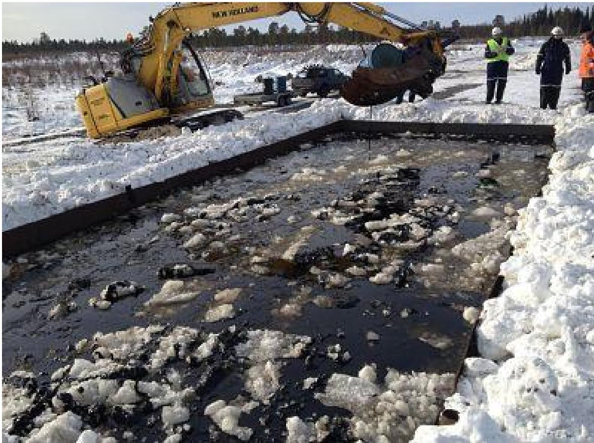
Figure 17 Test fields: each pool contained seawater, oil, ice block and snow in a predefined manner.
