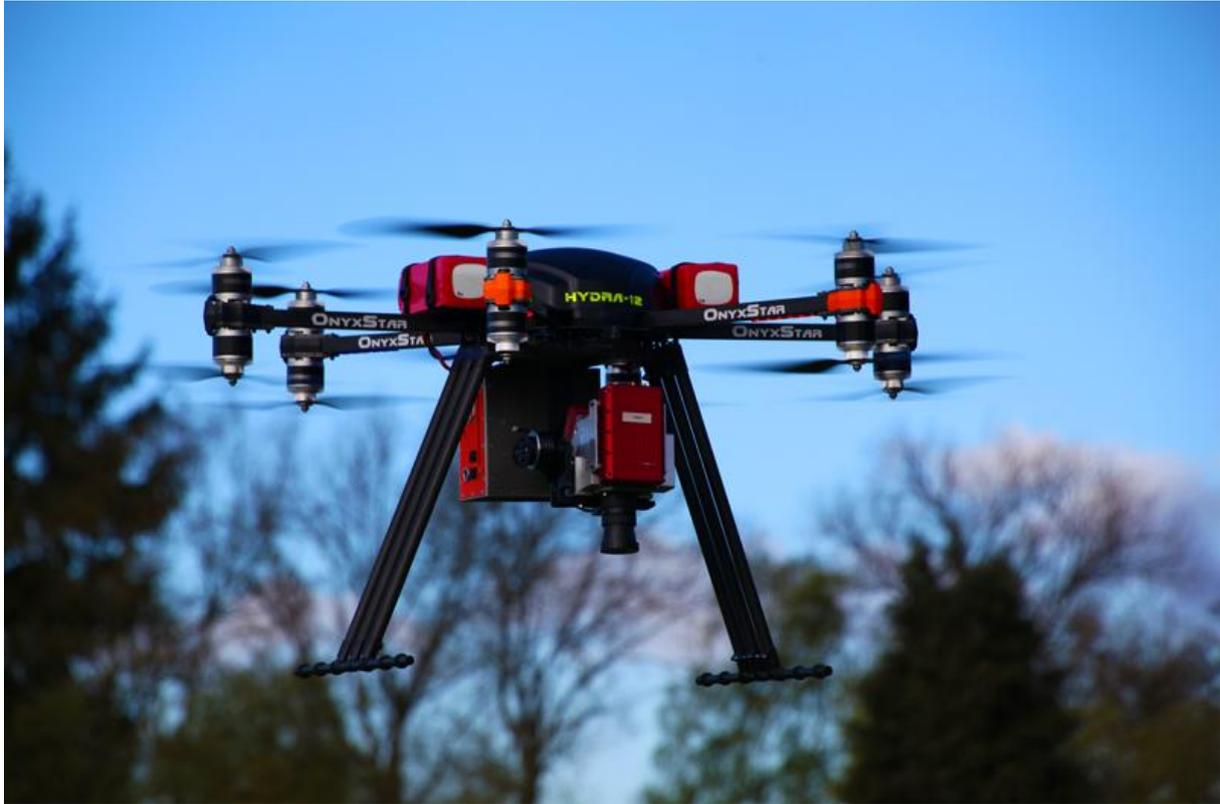
Figure 13 Hyperspectral camera embedded on OnyxStar HYDRA-12 UAV from AltiGator
