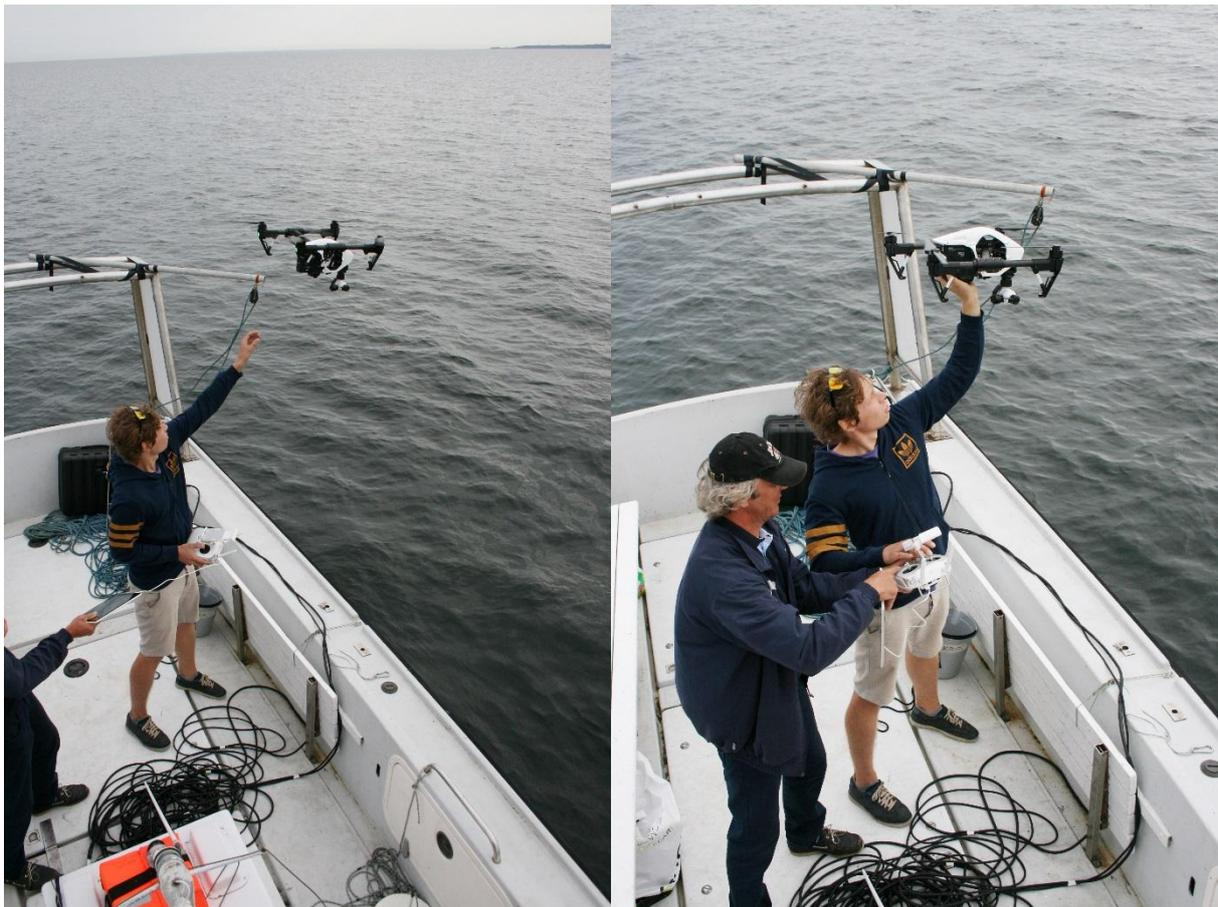
Figure 6 Operating the DJI Inspire 1 drone from a small vessel. As there was lack of landing space on board such a small vessel, the hand landing of the UAV was performed. Left panel shows preparations for hand landing – trying to keep the drone as steady as possible. Small drift from the waves and wind complicated the process. Right panel shows successful catching of Inspire 1 from the air.
