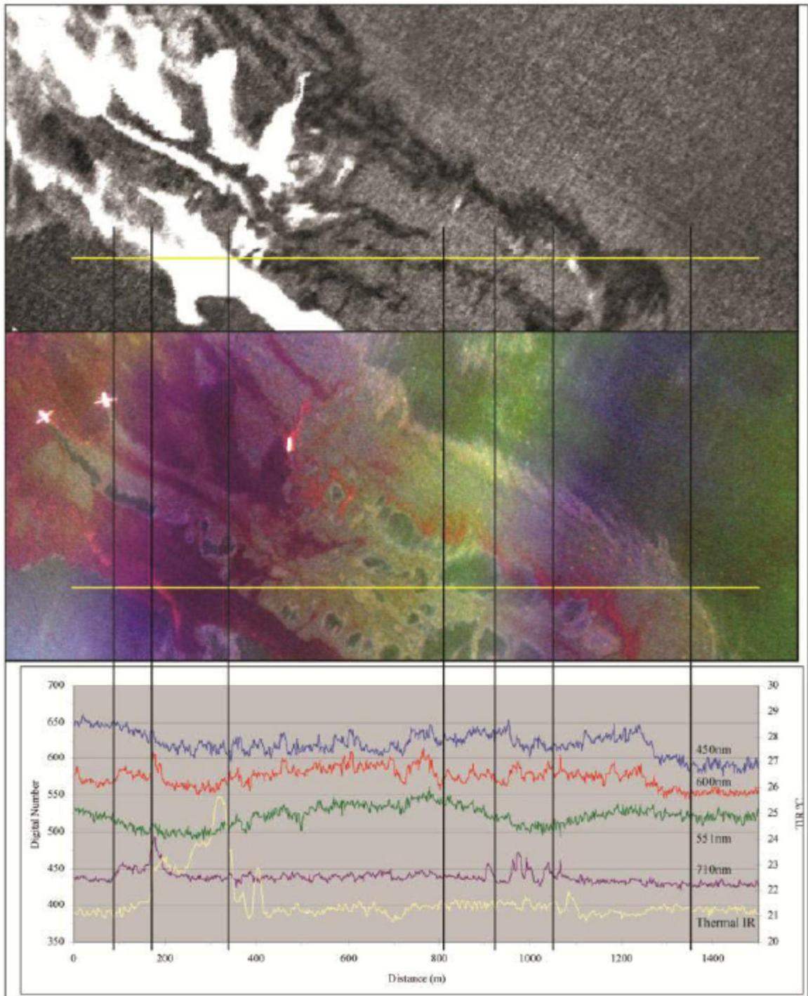
Figure 12 Thermal IR (top) and 450, 551 and 600nm color rendition of a large area of emulsified oil during the Deep Water Horizon spill as imaged by Ocean Imaging's aerial system. The graphs on the bottom show spectral reflectance/emission profiles along the yellow transect line. The thickest emulsions show the highest heat emission (white areas in top image) while thinner emulsions appear cooler (darker) than surrounding water due to petroleum's lower emissivity properties. [15]
