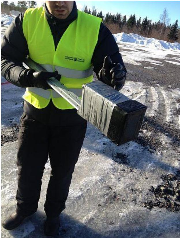
Figure 26 Hyperspectral camera inside the insulation box.
