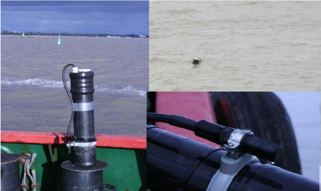
Figure 39 On-line buoy for measuring Total Suspended Matter (TSM)
