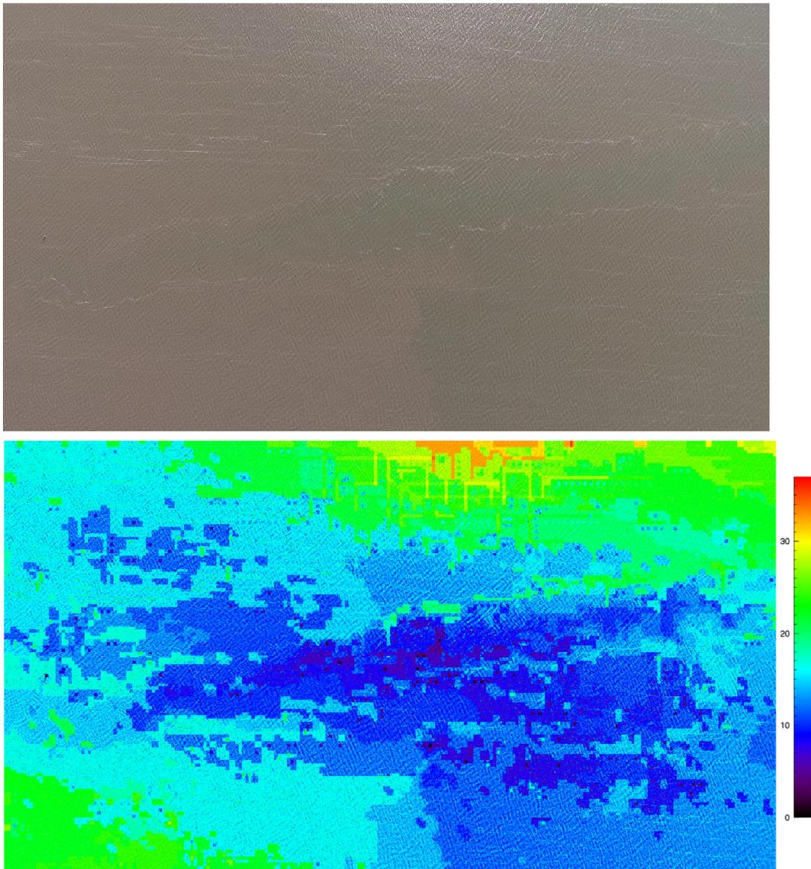
Figure 42 Example from 06 October 2015 07:00 UTC above and TSM concentration calculated from the image data. Measured TSM concentration was between 20.4 – 31.2 mg/l, which well agrees with buoy data (Fig. 40).
