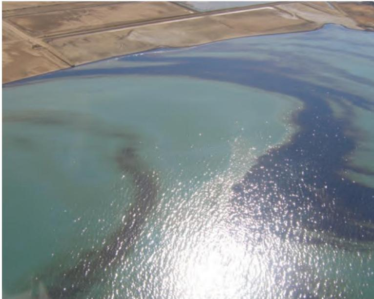
Figure 10 Light reflection off the sea can sometimes be a problem when taking aerial photographs; UV and polarizing filters may help to sharpen the visual definition of oil [14]
