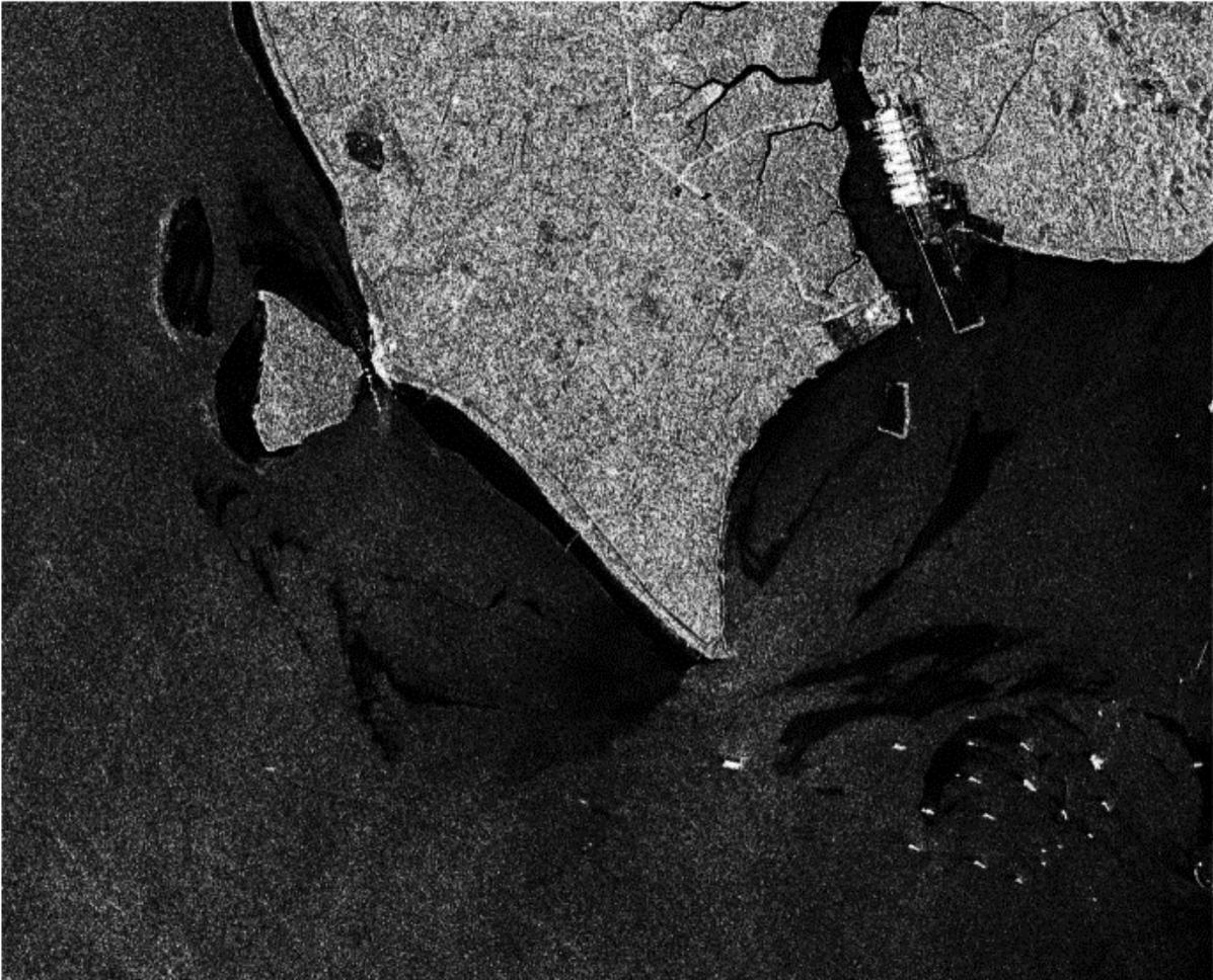
Figure 14 SAR (Synthesized Aperture Radar) image (RADARSAT-1) of oil spill in Strait of Malacca [17]
