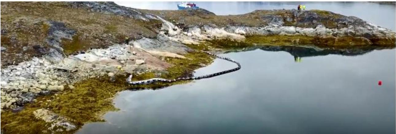
Figure 2. Image of the bay for the on-shore *in situ* oil burning experiment with the fire booms (footage from the video “Combat of oil spills in Arctic waters - in situ burning experiments, Greenland. Summer 2017. GRACE” <https://youtu.be/51ieM7h7ykM>)
