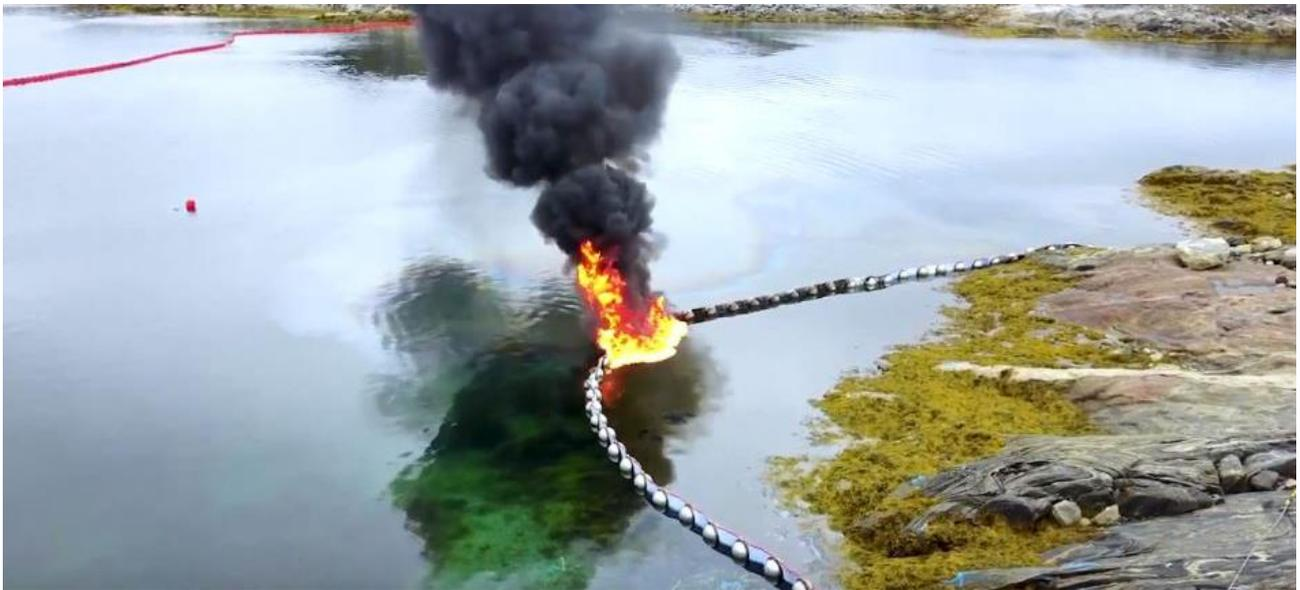
Figure 3. Image of the on-shore *in situ* burning of naphtenic North Atlantic crude oil after the fire was ignited. (footage from the video “Combat of oil spills in Arctic waters - in situ burning experiments, Greenland. Summer 2017. GRACE” <https://youtu.be/51ieM7h7ykM>)
