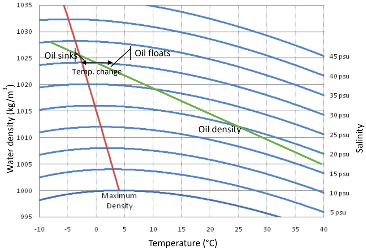
Figure 8 Water density as a function of temperature and salinity. Oil density as a function of temperature.
