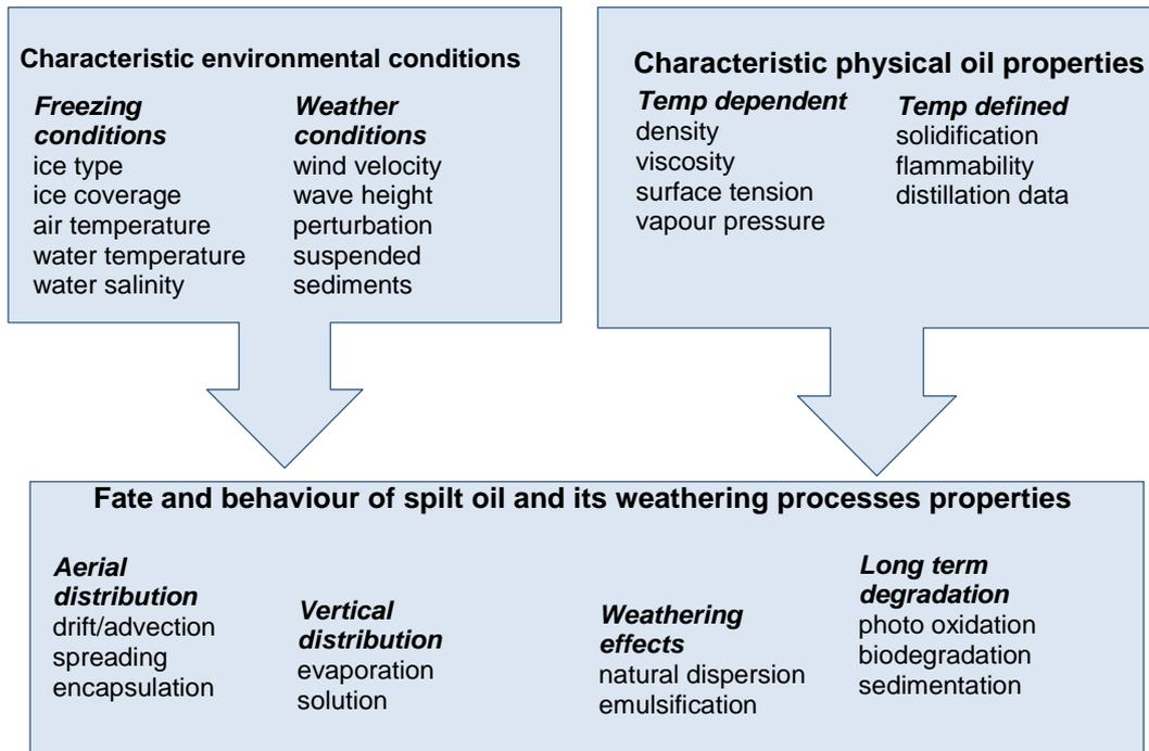
Figure 5. Box scheme: Schematic rationale on influencing factors/parameters governing the fate and behaviour on oil spills in water and ice.
