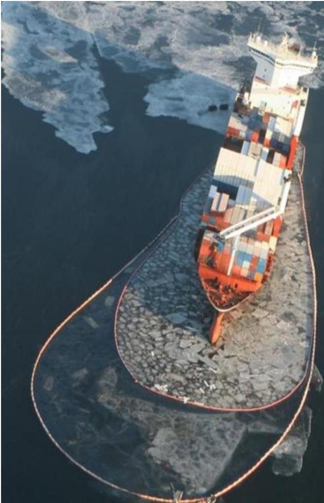
Figure 9 Containment booms around the grounded Godafoss in February 2011.
