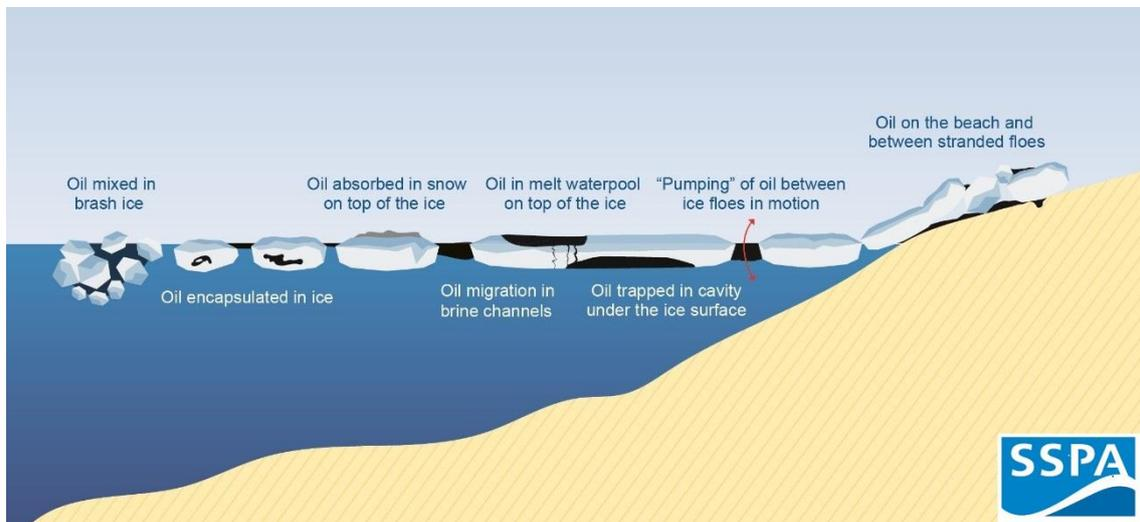
Figure 6. Known varieties of appearance of spilled oil in ice condition (Illustration: SSPA Sweden AB).
