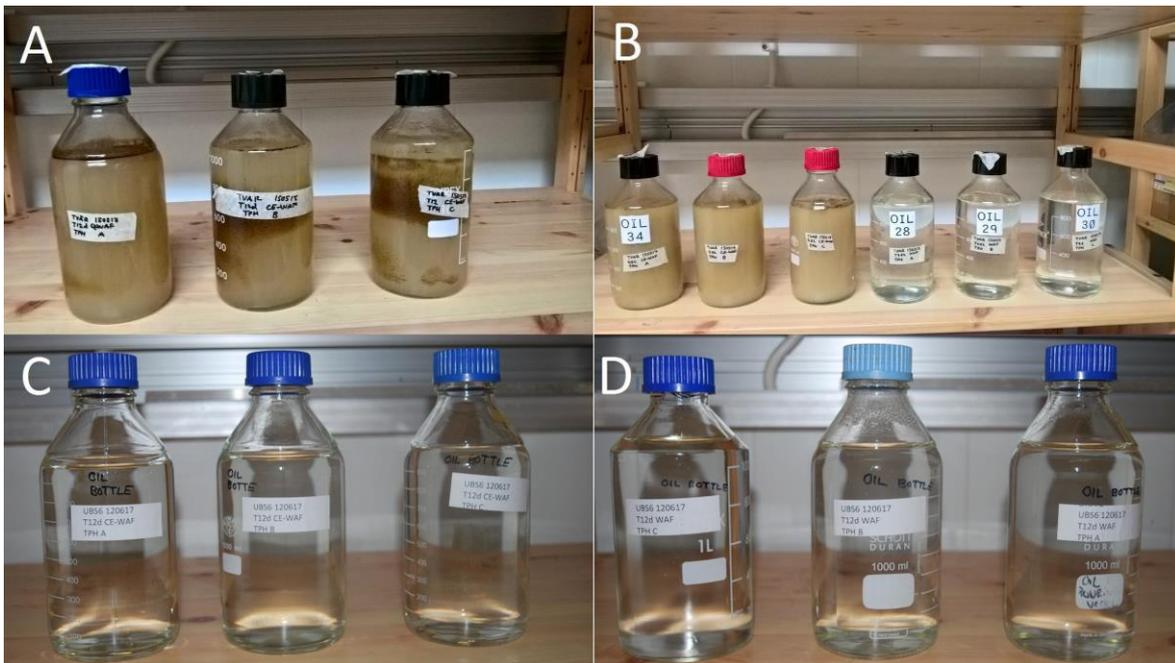
**Figure 5.** Microcosm bottles with different treatments from the two experiments. Pictures A and B are from the first experiment with undiluted WAF (only oil) and CE-WAF (oil and dispersant), bottles in picture A are from CE-WAF treatment and in picture B from CE-WAF and WAF treatments. Pictures C and D are from the second experiment, bottles in picture C are from CE-WAF treatment (diluted 1:1000) and in picture D from WAF (diluted 1:1) treatment.
