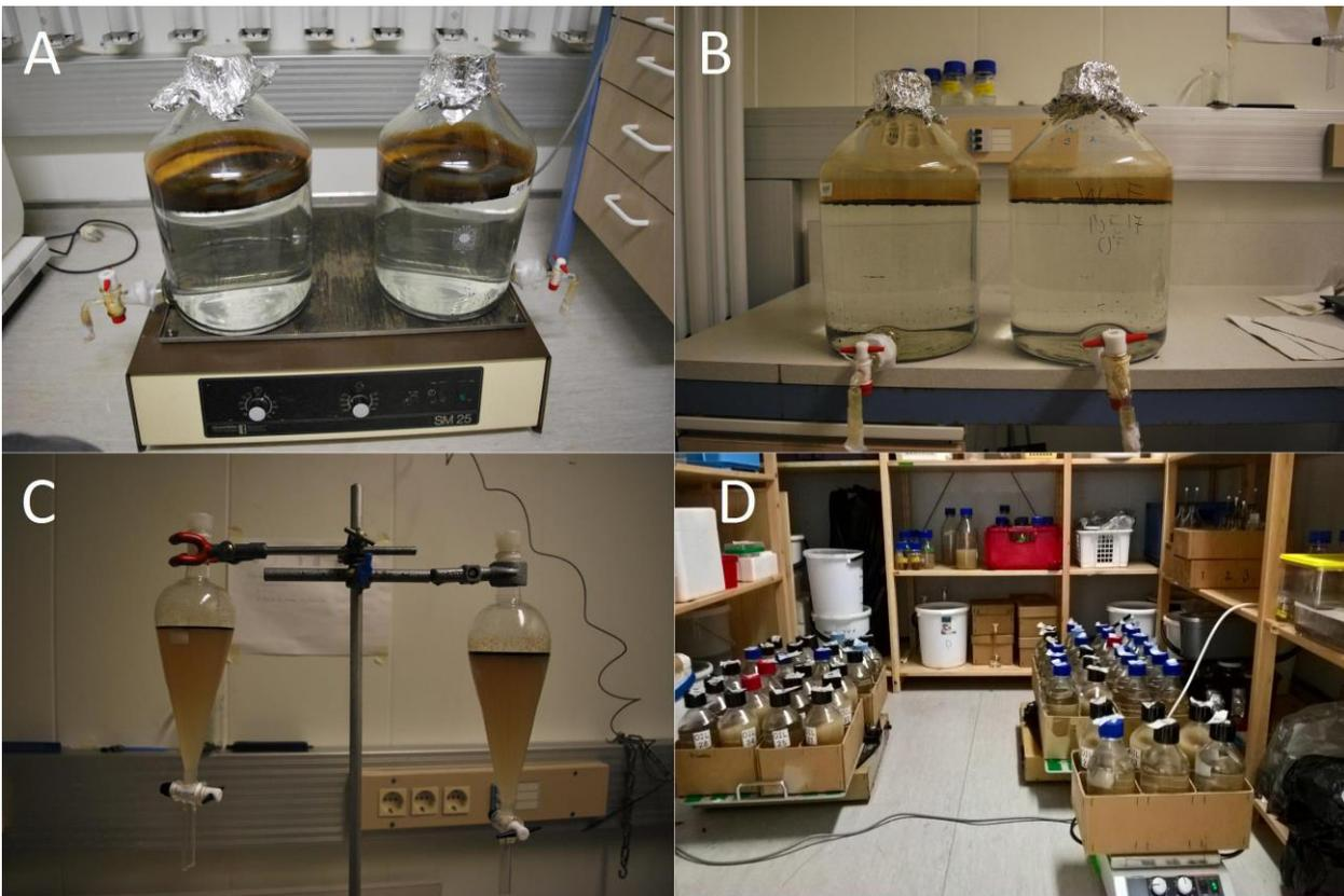
**Figure 3.** Different steps of WAF (crude oil) and CE-WAF (crude oil and dispersant) preparations for the microcosm experiments. Picture A: shaking of WAF bottles. Pictures B and C: settling of WAF and CE-WAF before bottling. Picture D: filled microcosm bottles in shakers.
